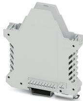
DIN rail housing, Lower housing part with metal foot catch, with FE contact, tall design, with vents, width: 22.6 mm, height: 99 mm, depth: 107.3 mm, color: light grey (7035), cross connection: integrated bus connector, number of positions cross connector: 10+2, Bus connector: 10 parallel contacts, 2 serial contacts
