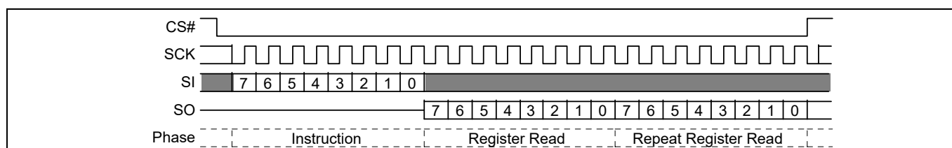
Figure 56 DLP Read (DLPRD) command sequence
